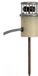
Figure 3.6. A modified Windtronic 2 anemometer as used to measure wind speed at ground level within the environmental treatments.
